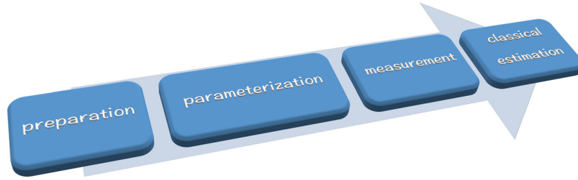
Figure 1. Schematic of a complete quantum metrological process, which contains four steps: (1) preparation of the probe state; (2) parameterization; (3) measurement; (4) classical estimation.
